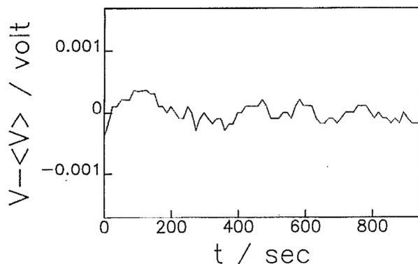
FIG. 3. Fluctuation of the output voltage ( $V$ ) around the average value ( $\langle V \rangle$ ) in our ( $2f$ - $2f$ ) design, which is caused mainly by the detector itself and not by the laser beam drift (see text for the detail).
