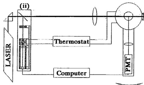
FIG. 2. Schematic of the incorporation of our differential refractometer into a laser light-scattering spectrometer.
