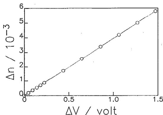
FIG. 4. Refractometer calibration curve obtained by using a set of NaCl solutions ranged from  $0.1$  to  $3.5$  g NaCl/100 g water, which corresponds to a range of  $\Delta n$  from  $\sim 2 \times 10^{-4}$  to  $\sim 6 \times 10^{-3}$  RI units. The circles represent the measured data and the line a least-squares fit.  $\Delta n/\Delta V = 3.92 \times 10^{-3} \text{ V}^{-1}$ .
