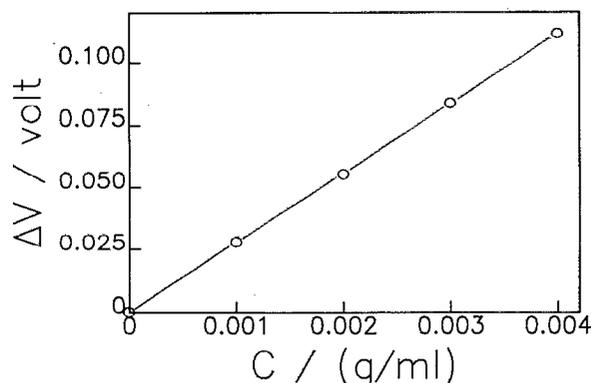
FIG. 5. Plot of the output voltage ( $\Delta V$ ) vs polymer concentration ( $C$ ) for polystyrene in toluene at  $\lambda_0 = 632$  nm and  $25^\circ\text{C}$ . The circles represent the measured data and the line a least-squares fit.  $\Delta V/C = 27.9 \text{ V/(g/ml)}$ .
