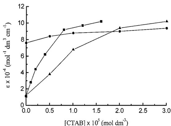
**Figure 4.** Variation of the molar absorptivity at 680 nm for **1** ( $\blacktriangle$ ), **2** ( $\blacksquare$ ), and **3** ( $\bullet$ ) ( $1.0 \times 10^{-5}$  mol dm<sup>-3</sup>) with concentration of CTAB.
