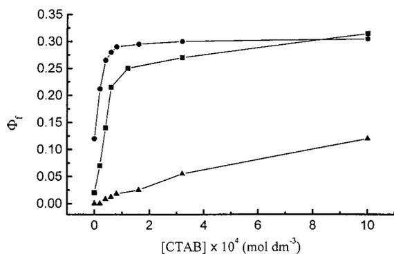
**Figure 5.** Variation of the fluorescence quantum yield of **1** ( $\blacktriangle$ ), **2** ( $\blacksquare$ ), and **3** ( $\bullet$ ) in water ( $2.0 \times 10^{-5}$  mol dm<sup>-3</sup>) with concentration of CTAB.
