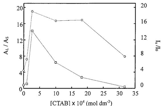
**Figure 9.** Plots of the peak area ratio ( $A_L/A_S$ ) ( $\square$ ) and the normalized scattered light intensity ( $I_s/I_0$ ) ( $\circ$ ) vs the concentration of CTAB. [**2**] =  $1.0 \times 10^{-4} \text{ mol dm}^{-3}$ .
