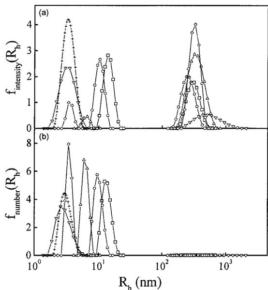
**Figure 8.** (a) Intensity- and (b) number-weighted distribution of the hydrodynamic radius of the **2**/CTAB complexes at a fixed concentration of **2** at  $1.0 \times 10^{-4} \text{ mol dm}^{-3}$  in  $0.01 \text{ mol dm}^{-3}$  NaBr aqueous solutions. [**2**]:[CTAB] = 1:0 ( $\square$ ), 1:1 ( $\circ$ ), 1:2.6 ( $\triangle$ ), 1:32 ( $\nabla$ ); + denotes pure CTAB.
