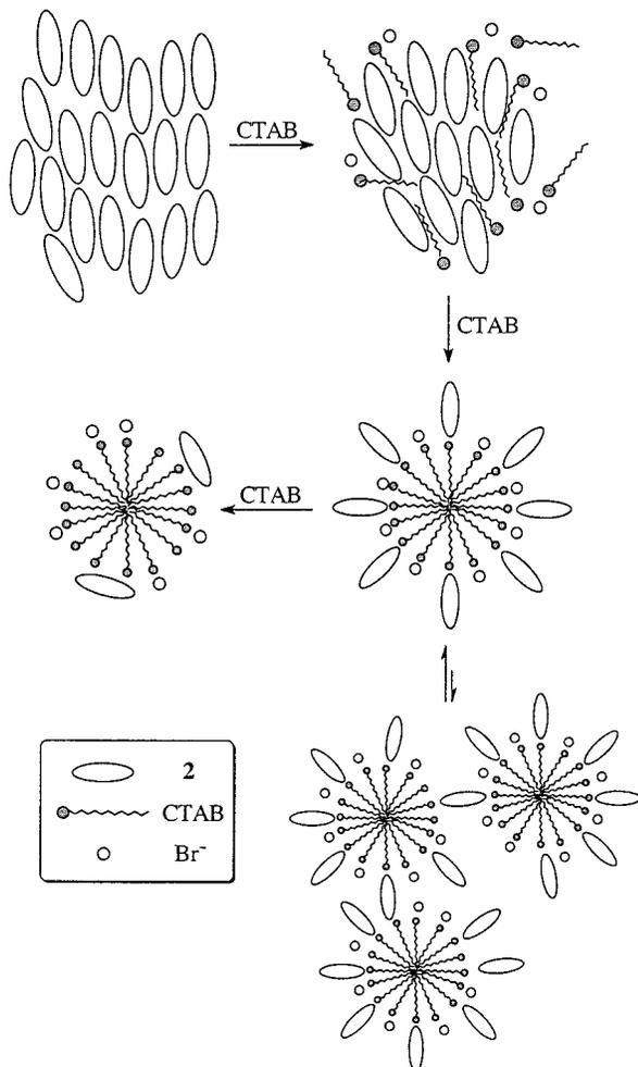
**Figure 10.** A schematic diagram showing the structural changes for the 2/CTAB complexes upon addition of CTAB.
